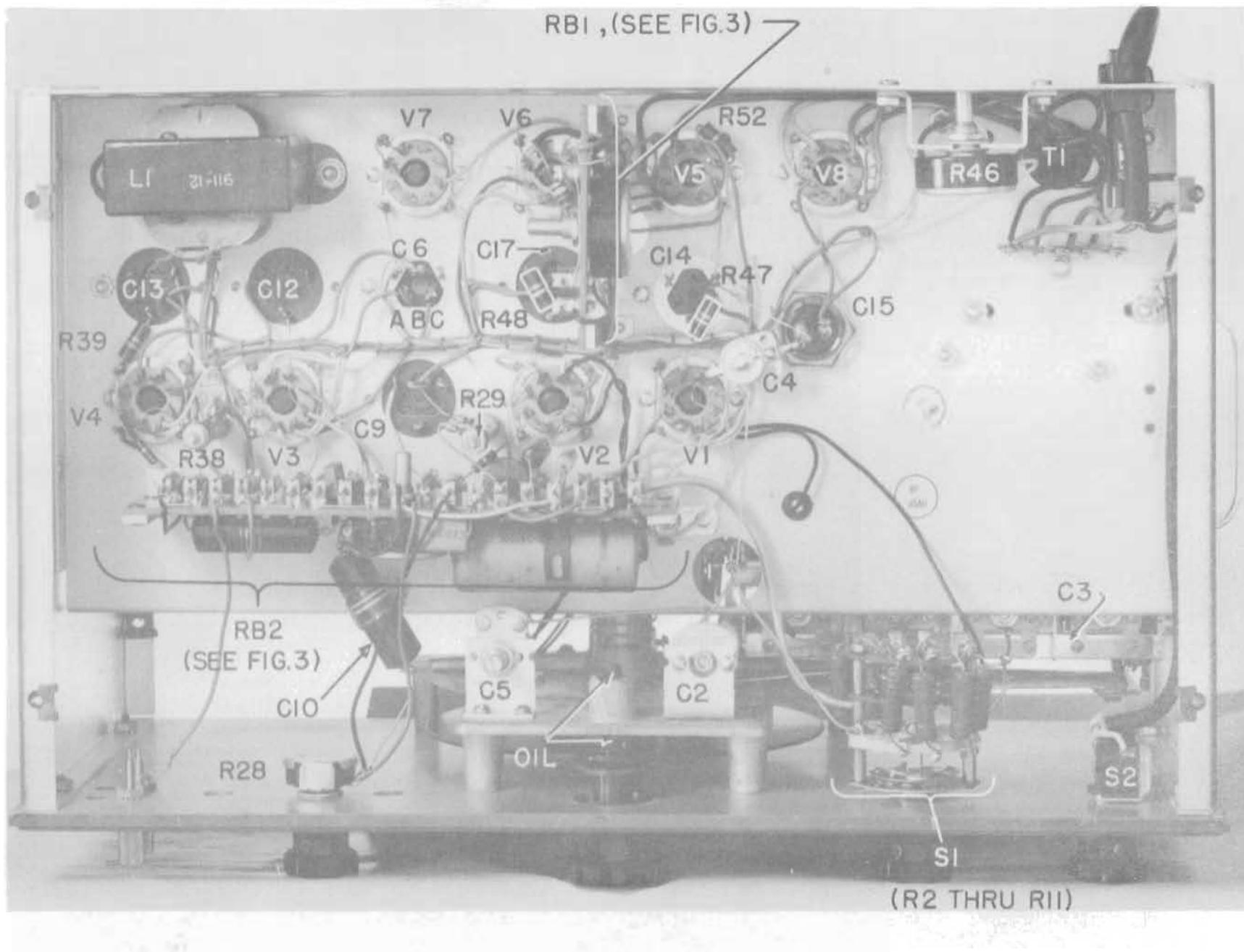
Fig. 2. Model 200H Bottom View Bottom Plate Removed
